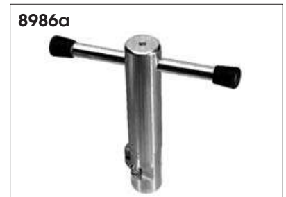
Chamfering device for removing the aluminium from stabi pipes as preparation for welding saddles
