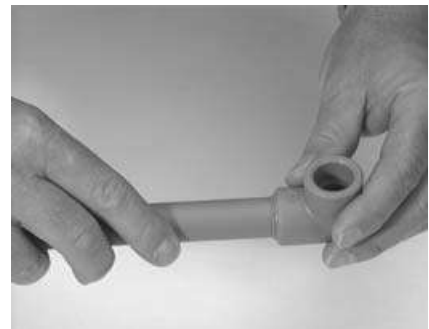
6. Adapt and join pipe and fitting within the max. allowed period without turning the parts against each other.
