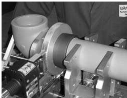
Fig. 9 Move the machine slides with the hand wheel, warmup the pipe and the fitting in the welding tools
