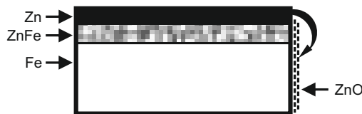
Protection of cut edges with zinc coatings.
